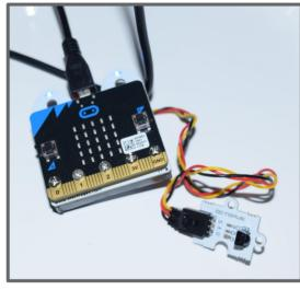
Connect an IR sensor to the micro:bit with alligator clips or an extension board. The photo shows ring:bit with IR sensor attached to pin 1.
