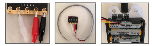
Drag the *attach LED NeoPixel* block to the scripting area. Input both the number of NeoPixels on your strip and the pin to which the strip is connected, then run it.
