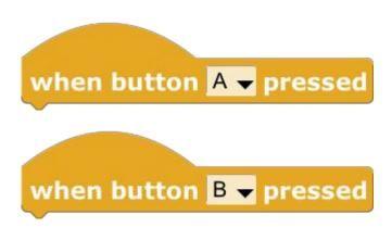
Try these scripts to make the buttons on the micro:bit turn the LED display on and off!
