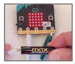
The **read analog pin** block senses voltage. A new battery outputs about 1.6 volts, which reports about 520. Even a dead battery outputs about 0.9 volts, which reports 290. Use this script to see the number from the **read analog pin** block.
