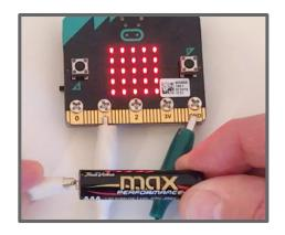
The **read analog pin** block senses voltage. A new battery outputs about 1.6 volts, which reports about 520. Even a dead battery outputs about 0.9 volts, which reports 290. Use this script to see the number from the **read analog pin** block.
