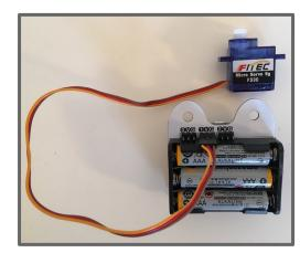
**NOTE:** The micro:bit needs extra power to run servos. Be sure to attach batteries or use an extension board that provides extra power.
